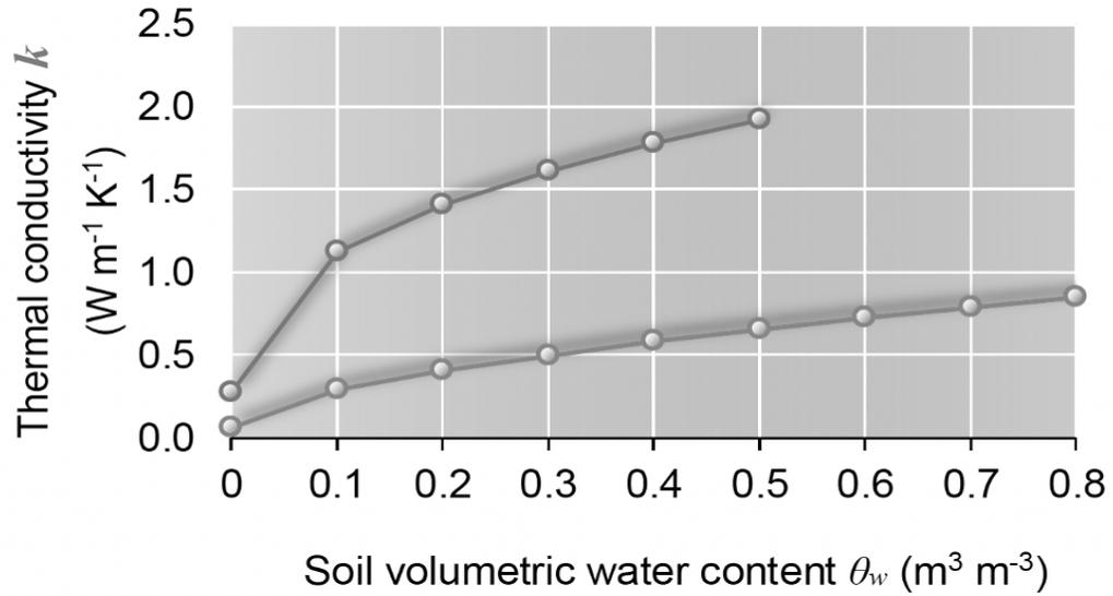
(a) Indicate which line corresponds to the mineral soil and which one corresponds to the organic soil. Note that you can label them directly on the graph. [4]
