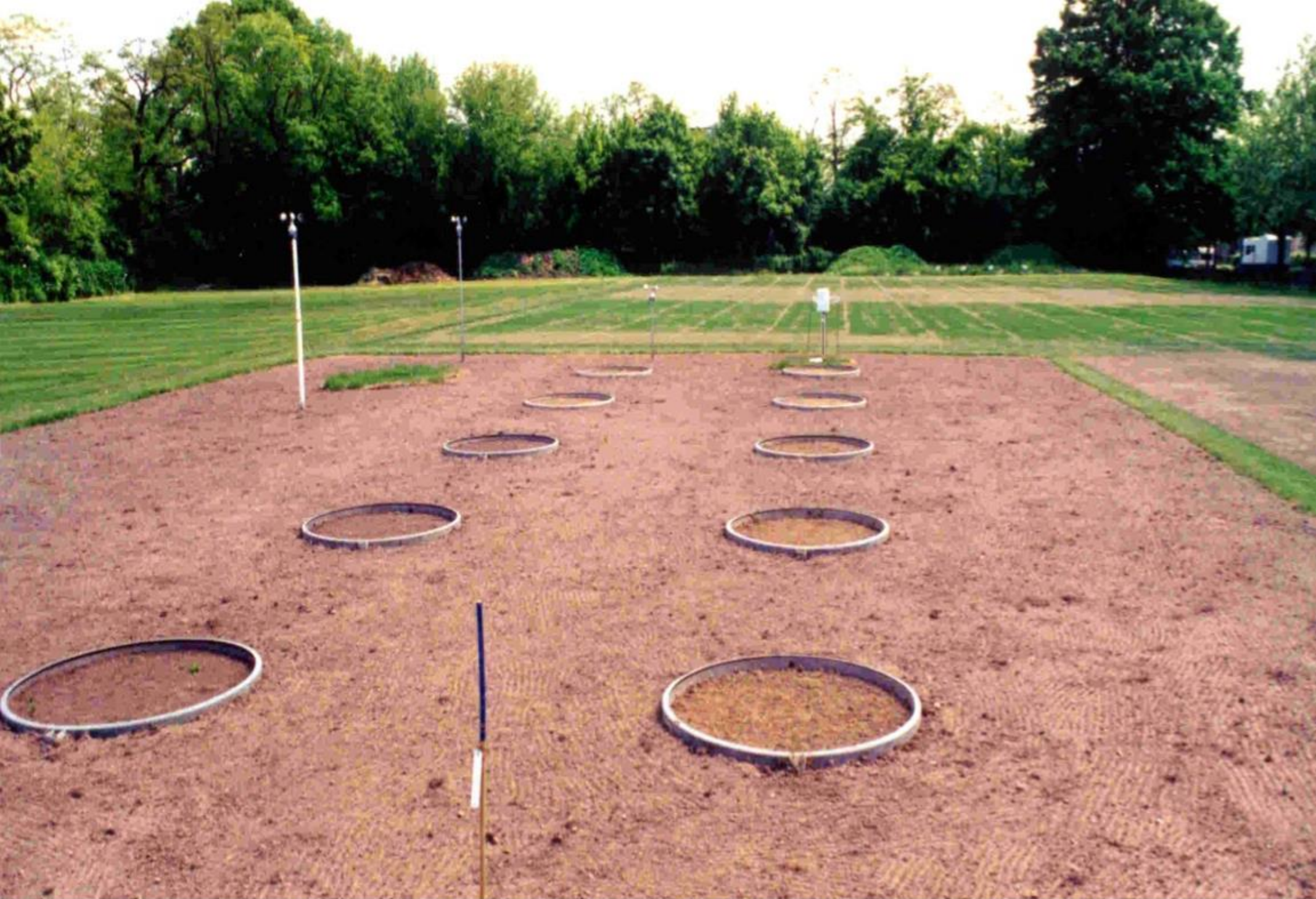
Lysimeter array over bare soil (Photo: TU Berlin, Thomas Zenker)
