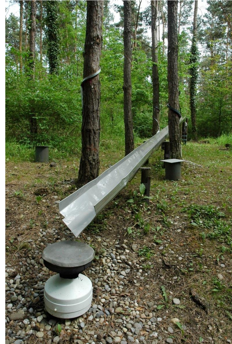
Measuring throughfall of precipitation in a forest using guttering and a rain gauge
