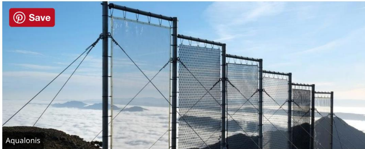
Mesh billboards can capture tiny fog droplets in mountainous regions (Image credit: Aqualonis)
