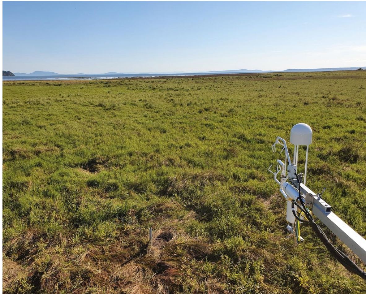
Measurement of convective fluxes using the EC technique at a salt marsh in Boundary Bay, Delta, BC (Photo: Tzu-Yi Lu, UBC)
